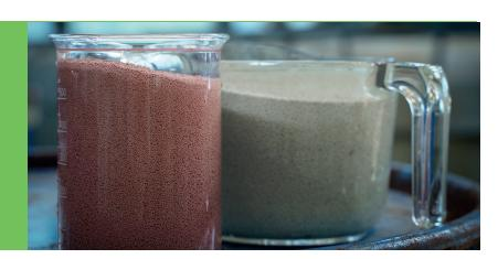
With the production and distribution of regenerable adsorbent materials we remove arsenic, fluorine, boron, iodine, iron, manganese, ammonia, and sodium from the water. As a bulk filter media this is an excellent solution for water utilities and water technology companies and for some industrial water management providers.
